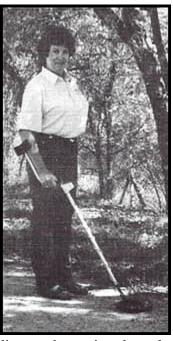
The pole length is adjusted by depressing the spring buttons and extending or shortening the pole until the spring buttons click into the set of holes that give you the most comfortable pole length.
