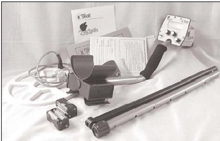
Assembling the DeLeón is simple and requires no special tools. Just install the battery packs, mount the searchcoil on the lower pole assembly, connect the pole assemblies together, wrap the excess cable around the pole and plug the cable into the control housing. Finally, adjust the pole length and searchcoil angle and you're ready!
