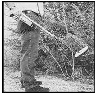
You must lift your coil straight up. Do not swing it like a pendulum.
