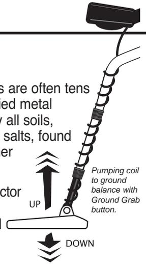
When the detector is calibrated to the soil, the result will be deeper target detection, quieter operation, and more accurate target identification.
