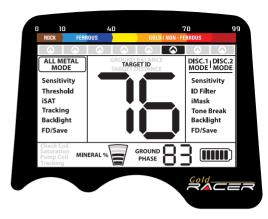
If no button is pressed for a while after selecting a setting or changing its value, the selection cursor automatically returns back to the selected mode. Pulling the trigger eliminates the waiting time.
