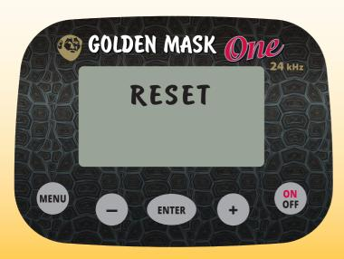
To turn off the detector, press and hold the ON/OFF button. A screen with HOLD TO TURN OFF will appear.
