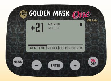
If you set the Iron Audio bar at the full-left position (-22), the detector works in All-Metal mode. This means the sound from all targets will be the same. You can still identify the target by the VDI number and the SpectrumVDI bars. In All Metal mode, the detector gains a little bit more depth, but this mode is good only on clean places with very few targets. Otherwise you will have to constantly look at the screen and this is not quite comfortable.
