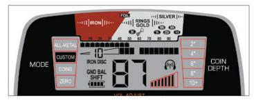
Ground Balance values above 75 increase in quarter-points of resolution. The above illustration indicates a Ground Balance value of 87.5. Above the solid numeral 87, each quarter-point of value is indicated by five blocks of pixels on the upper scale.
