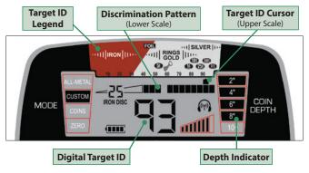
**Target ID Legend**—Works with the Target ID Cursor to indicate a target's probable identity, with Ferrous (iron) targets at the left, non-ferrous targets that are thin or have low conductivity in the middle, and thick or high conductivity targets (e.g. thick silver) at the right.
