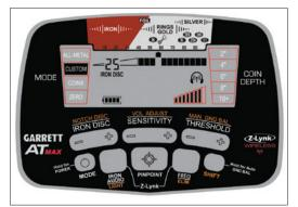
Note: Changes made to the Notch Discrimination pattern while in CUSTOM Mode will be retained when the detector is switched OFF. Changes made to all other modes will return to the factory settings when the detector is switched OFF and back ON.
