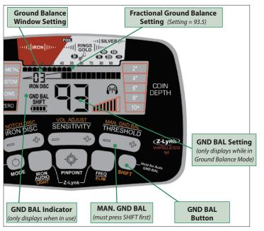
**GND BAL Button**—Hold the SHIFT button for Automatic Ground Balance or, for Manual Ground Balance, press and release SHIFT and then use the (+) and (-) MAN. GND BAL buttons.
