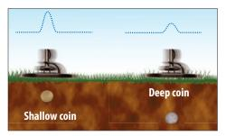
Example B: Notice the different target response provided by the *AT Max*'s proportional audio in regards to target depth. The shallow coin target offers a stronger signal, while the same-sized deep coin provides a softer signal.
