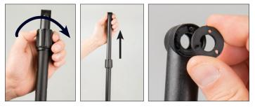
Connect searchcoil to stem as shown, and hand-tighten wing nut. Loosen upper camlock, depress the spring clip in the S-stem (containing control housing), and insert the S-stem through the upper camlock collar into the upper stem.
