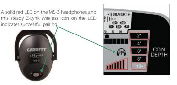
Once paired, if the headphone/receiver is switched off or moved out of range, the *AT Max* will search and attempt to reconnect to the receiver for 30 seconds, indicated by a flashing icon. If the connection is not reestablished during this time, the *AT Max* will switch off its wireless transmitter. It will be necessary to switch the *AT Max* off and then on again to initiate a new 30-second search.
