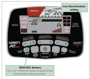
**Iron Masking:** To prevent an iron object from "masking" out the signal of an adjacent good target, use just enough discrimination to barely reject the iron trash (e.g. small nail, as seen in Illustration 1). This will allow you to detect the coin and nail together (see Illustration 2) and not miss/mask a good target.
