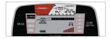
While in the ALL METAL Mode, the *AT Max* will respond to the entire range of conductive and magnetic properties encountered, including ground responses. The user is continuously hearing what the searchcoil is "seeing" in the ground. Therefore, it is essential to be properly ground balanced while operating in the ALL METAL Mode. Naturally occurring minerals in the soil must be canceled out during the ground balance procedure in order to detect only the signals from metal objects.
