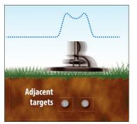
Example A: Adjacent targets can often produce a single strong signal with many metal detectors. The fast recovery of the *AT Max*, however, will provide two peaks of audio response to these adjacent coins. These multiple audio responses provide the experienced user with more target information.
