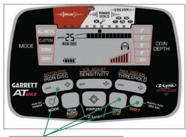
Press SHIFT, then use the NOTCH DISC buttons to position the Target ID Cursor above the pixel you wish to eliminate (see illustration). Use the ELIM button to delete this pixel from the Lower Scale (see below). This item is now rejected.
