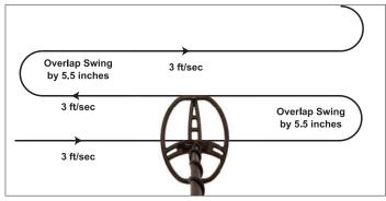
In order to fully search an area, overlap the swings of your searchcoil by half the length of the coil (about 5.5 inches). Sweep the searchcoil in a straight line or with a slight arc at a sweep speed of about 3 ft/sec.
