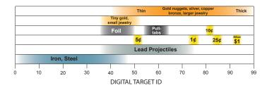
Target ID can vary widely based upon the target's size and thickness because small, thin pieces of metal cannot conduct electrical current as well as thicker pieces of metal. In addition, mineralized soils can cause Target ID errors, especially for small targets.
