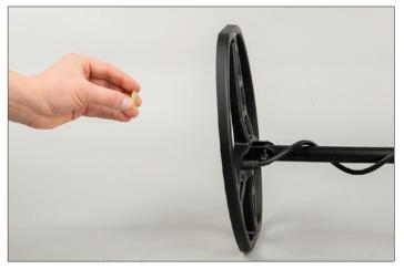
For bench testing, place the searchcoil on a flat, stable, non-metallic surface that is several feet from other metallic objects.
