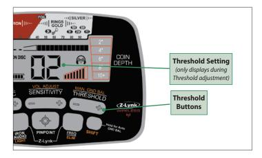
Threshold is the constant background "hum" that is added to the target response. Press a Threshold button once to display the current setting. Press the (+) or (-) Threshold buttons again to select from 33 levels, ranging from -9 up to +23.
