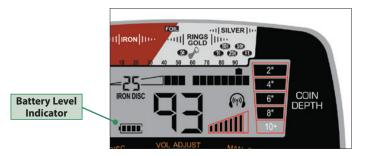
Four bars indicate fully charged batteries. Replace batteries when there is only one bar remaining. The detector will maintain full performance until the batteries need to be replaced. NiMH rechargeable batteries may be used, but may have a shorter life per charge. You can expect 15-25 hours of operation without wireless headphones, and 10-20 hours with wireless headphones, depending on battery type and quality.
