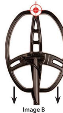
Once the target signal drops off (both audibly and on the LCD meter), shallow targets should be located immediately in front of the searchcoil's tip (see *Image B*). Deep targets will be under or just inside your searchcoil's tip. This is because the conical shape of the searchcoil's detection field begins bending in slightly as the depth increases.
