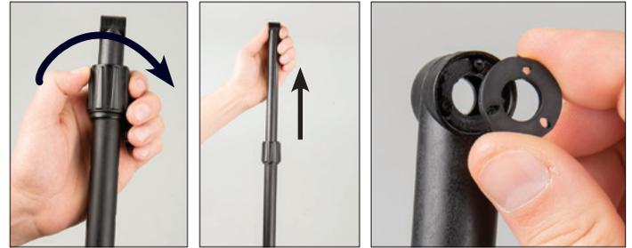
Connect searchcoil to stem as shown, and hand-tighten wing nut. Loosen upper camlock, depress the spring clip in the S-stem (containing control housing), and insert the S-stem through the upper camlock collar into the upper stem.
