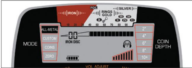
While in the ALL METAL Mode, the *AT Max* will respond to the entire range of conductive and magnetic properties encountered, including ground responses. The user is continuously hearing what the searchcoil is "seeing" in the ground. Therefore, it is essential to be properly ground balanced while operating in the ALL METAL Mode. Naturally occurring minerals in the soil must be canceled out during the ground balance procedure in order to detect only the signals from metal objects.
