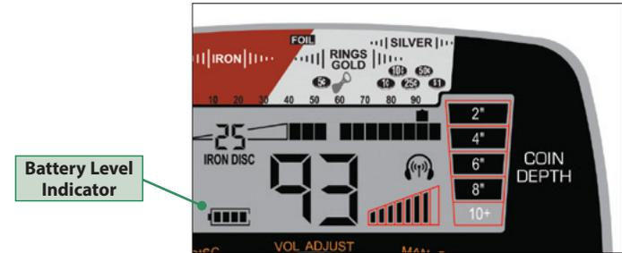
Four bars indicate fully charged batteries. Replace batteries when there is only one bar remaining. The detector will maintain full performance until the batteries need to be replaced. NiMH rechargeable batteries may be used, but may have a shorter life per charge. You can expect 15-25 hours of operation without wireless headphones, and 10-20 hours with wireless headphones, depending on battery type and quality.
