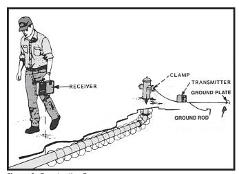
Figure 9. Conductive Trace
