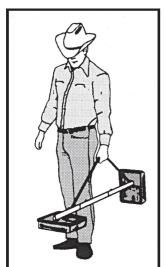
**Figure 6.** Handle strap: Using the handle strap increases depth; however, it may be difficult to tune the GEMINI-3 this close to highly mineralized ground.
