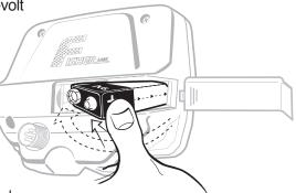
side of the Control Housing. Slide the battery door to the side to remove. Insert battery (*see illustration*). Close battery door. When it is time to replace the battery, simply pull up firmly on the end of the battery.
