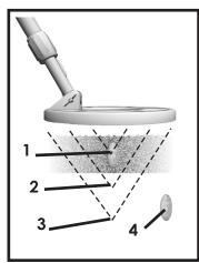
Figure 7. Searchcoil Detection Pattern
