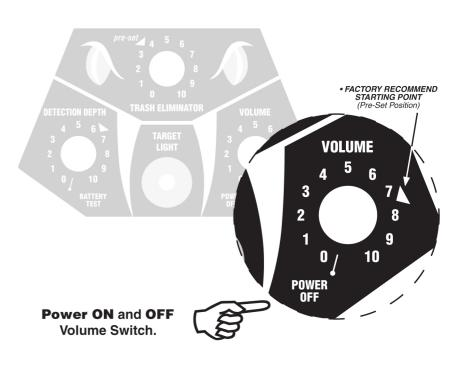
To operate and turn on the **Cobra Beach Magnet** simply turn the **Power/Volume Control** fully clockwise. Turning this same control counterclockwise will lower the headphone volume.
