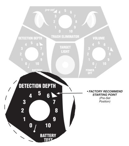
By starting out at the Pre-set point the **COBRA Beach Magnet** is set at the **normal detection depth range**. The normal range is good for most soil conditions, but by increasing this control clockwise to the maximum position you will get better depth on older coins. This control is extremely helpful in elimination false signals caused by high minerals. If you are experiencing false signals you should decrease this control until these signals are minimized.
