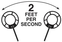
**3. Correct arm position.** Adjust the lower stem so that your arm is hanging in a comfortable position by your side with the coil about 1 inch off the ground.
