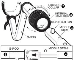
4 Insert the MIDDLE STEM into the S-ROD, with the SILVER BUTTON pointed upward
