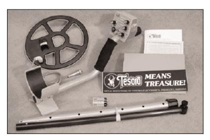
Assembly of the Vaquero is simple and requires no special tools. Just install the battery, mount the searchcoil on the lower pole assembly, connect the pole assemblies together, wrap the excess cable around the pole and, plug the cable into the control housing. Finally, adjust the pole length and searchcoil angle and you're ready!
