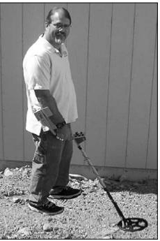
The pole length is adjusted by loosening the pole lock, then depressing the spring buttons and extending or shortening the pole until the spring buttons click into the set of holes that give you the most comfortable pole length.
