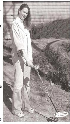
To adjust the searchcoil angle, simply loosen the searchcoil thumb nut slightly and move the searchcoil into the desired position. Tighten the searchcoil thumb nut by hand so that the searchcoil will hold in place.
