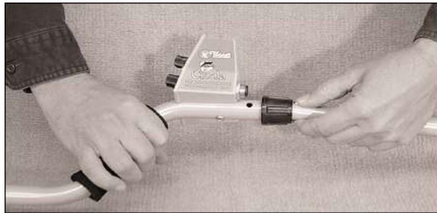
6. Slide the lower pole into the middle pole until the spring buttons click into the first set of adjustment holes. Turn pole lock to tighten the assemblies into place.
