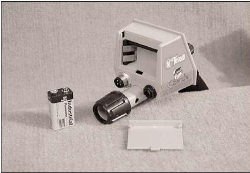
To install or replace the battery, first make sure the SENSITIVITY control is set to POWER OFF—turned completely counterclockwise past the “click.” Remove the battery door from the back of the control housing. Do this by pressing your thumb firmly on the louvered square—at the bottom of the battery door—and sliding the battery door upward in the direction of the arrow.
