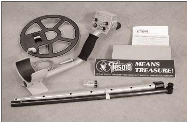
Assembling the Cibola is simple and requires no special tools. Just install the battery packs, mount the searchcoil on the lower pole assembly, connect the pole assemblies together, wrap the excess cable around the pole and plug the cable into the control housing. Finally, adjust the pole length and searchcoil angle and you're ready!
