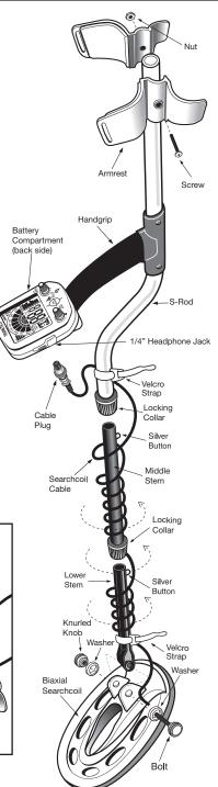
Caution: Forcing in MIDDLE STEM with CAM LOCK raised may form a burr on cam lock. If this happens, remove burr with knife to allow insertion.
