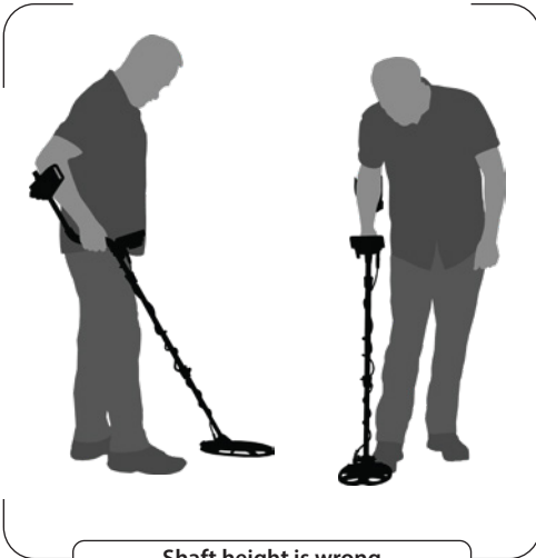
Shaft height is wrong
