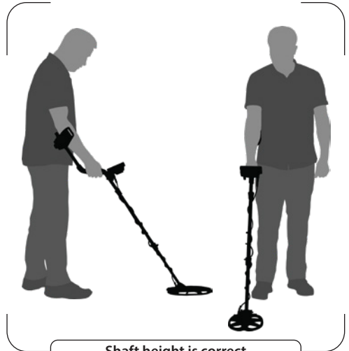
Shaft height is correct
