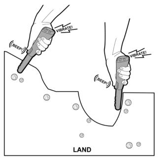
When using the Vulcan in the field it is recommended to shut the power off to conserve the battery when not being used. (The Vulcan has a built-in auto shutoff feature when left on and will shut off in approximately 5 minutes giving 4 long audible beeps before shutting off.) To turn on again, simply press and release the Power button.
