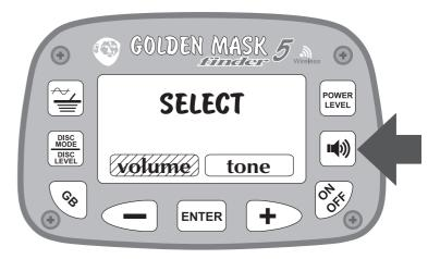
Now you will see a screen with number. By selecting the desired value, you change the sound volume. At every push of the button, you will hear a sound. When the sound volume matches your desired level, confirm with the ENTER button.
