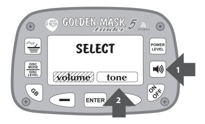
Then select the tone you want to change (for non-ferrous or ferrous targets) and select the desired frequency by pressing the - and + buttons. As usual, confirm your choice by pressing the ENTER button.
