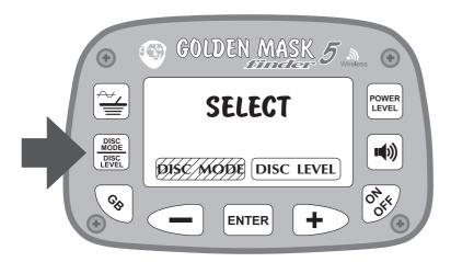
After you select and confirm the DISC MODE option, a selection screen with three options will appear - Mono, 2 and All, as shown on the next graphic.
