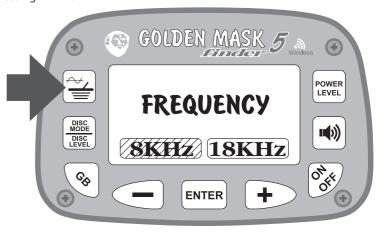
After you've selected the frequency and confirmed with the ENTER button, a screen with two options will appear. This is the so-called frequency shift. By selecting one of these two options, the working frequency changes slightly to avoid electromagnetic interference with similar devices or industrial electromagnetic fields. Select the desired value (I or II), the selected option is above the ENTER button, and confirm your choice with the ENTER.
