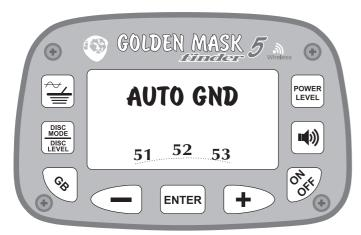
bottom-left corner of the control panel, then select the Auto option from the ground balance menu and confirm your choice with the ENTER button. A new screen will appear.
