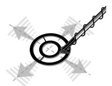
When pinpointing a target, try drawing an "X", as illustrated, over where the tone is induced.
