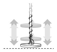
Move the GROUND control to the left-most position at which the detector DOES NOT beep while moving the coil up and down in a Yo-Yo fashion.
