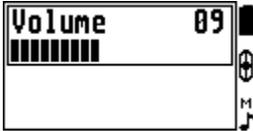
This option allows adjusting device sound volume to your own preference. External speaker turns off when the headphone jack is inserted into the slot on the front panel and this option allows adjusting headphone sound volume.
