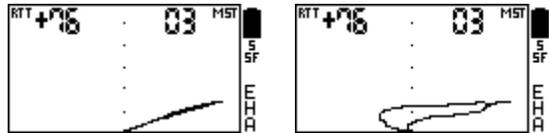
all similar devices. In both cases target VDI would be +57 +58. It is seen in hodograph shape only that in first case (left picture) the target is sure to be nonferrous. In second case (right picture) it is safe to say that there is a flat iron target under the coil, a piece of iron roof coating, fragment of a kettle, for example.
