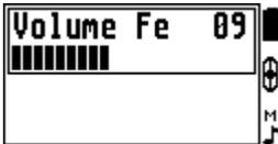
This option allows making separate adjustment of sound volume for iron only in order to increase comfort and reduce sound overflow in the "all metals" mode. But this may cause some reduction in sound descriptiveness. Adjust this setting for the sake of your convenience.
