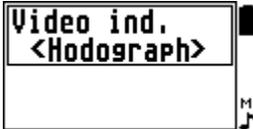
This option allows switching between types of data display on the main operating screen.
