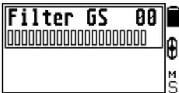
Option allows selecting false signal block-out level, signals caused by high conductivity of the ground (salty soil, sea beach etc).
