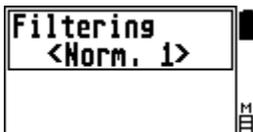
Search conditions imply presence or absence of such influencing factors as metal trash, rough plants, rugged ground surface (plowland). Selection of "Met. Trash" mode increases device operating speed as well as its ability to distinguish
