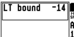
This option allows moving the sound border of **nonferrous** low tone (LT) to the iron sector by the required value.
