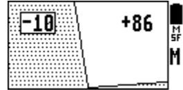
The discrimination range of your device is set up by the allowed width of the search sector (a VDI sector between left and right borders of the discriminator). When the discrimination mode is on your device will respond to objects with a VDI and hodograph located within the allowed response sector only.
