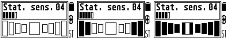
If the signal is too strong and continuous, the target is large and relatively close to the surface. Raise the coil to the level where the target is less responsive and you will be able to detect target contour in the ground by crossing passes.
