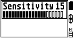
This option allows adjusting sensitivity of your device. You may change its value from 0 to 21. Remember, increasing device sensitivity you get search depth increase but it comes along with possible interference from power lines and false responses from the search coil bumping obstacles.
