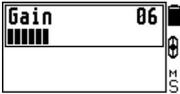
Option allows regulating search coil signal boost for the detection channel (Threshold tone) and identification channel (ST Sensitivity) simultaneously. Such setting may be used in extremely trashy areas, beaches etc, when there is no need in a great search depth, and distinction of objects located close to each other is more important.
