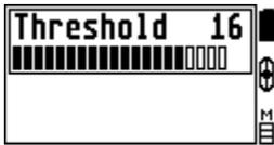
This option allows adjusting sensitivity (detection depth) of the threshold tone of your device. The threshold tone is a detection channel signal informing you of the metal object detected by the device. After detection and during search coil motion the sound volume of the threshold tone increases, the highest value is above the center of the target.
