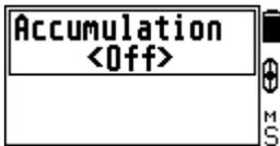
When the storage mode is "off" the display will show only the hodograph of the latest target identified by the device. Once the next target is identified, the previous hodograph is deleted. In the "auto" mode the display saves hodographs of the last three targets identified consequently.
