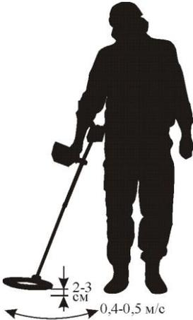
Try to avoid horizontal search coil jerks. Optimum scanning speed 40-50 cm/s. Each successive scan must overlap the previous one at least by a half.
